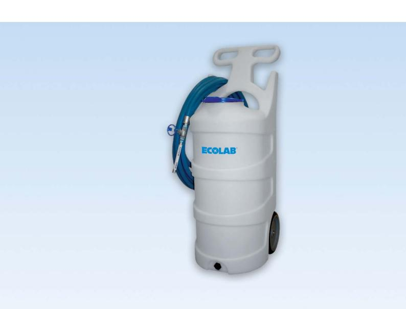
The new MobyFoam FI-20N mobile foam unit, with a tank capacity of 75 litres, offers an innovative and ergonomic solution for the cleaning of small areas in the food processing industry.
