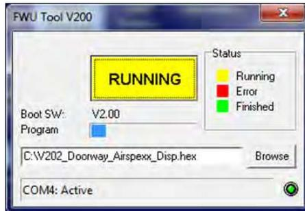
15. The progress bar "Program" must go to the end before the upgrade is complete (less than 1 minute)
