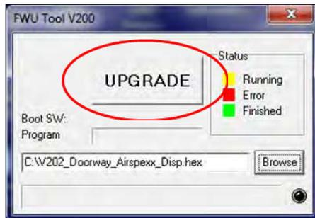
15. After a short while the FWU tool should start upgrading, the upgrade button should turn Yellow and change to "RUNNING"
