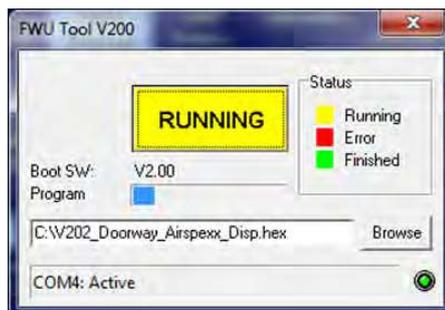
16. The progress bar "Program" must go to the end before the upgrade is complete (less than 1 minute)
