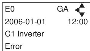
The error log stores up to 30 occurrences. When max. memory is reached, the errors will be deleted according to "First in" First out" principle.
