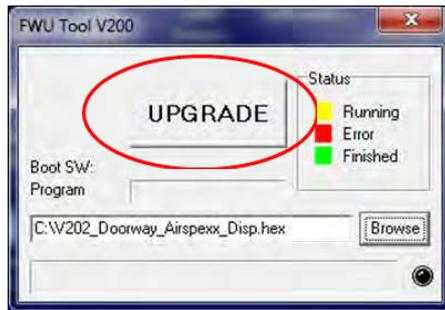
14. After a short while the FWU tool should start upgrading, the upgrade button should turn Yellow and change to "RUNNING"
