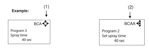
(1) When switched on the display will show an arrow symbol in the top right corner equivalent to the active navigation buttons on the Display Module.
